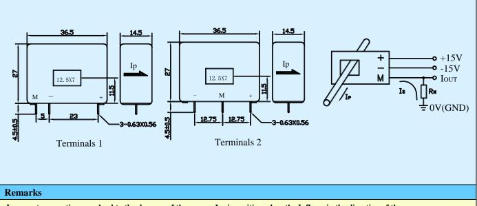
Incorrect connection may lead to the damage of the sensor.  $I_{SN}$  is positive when the  $I_P$  flows in the direction of the arrow. Dynamic performance (di/dt and response time) are best with a primary bar in the center of the through-hole.
