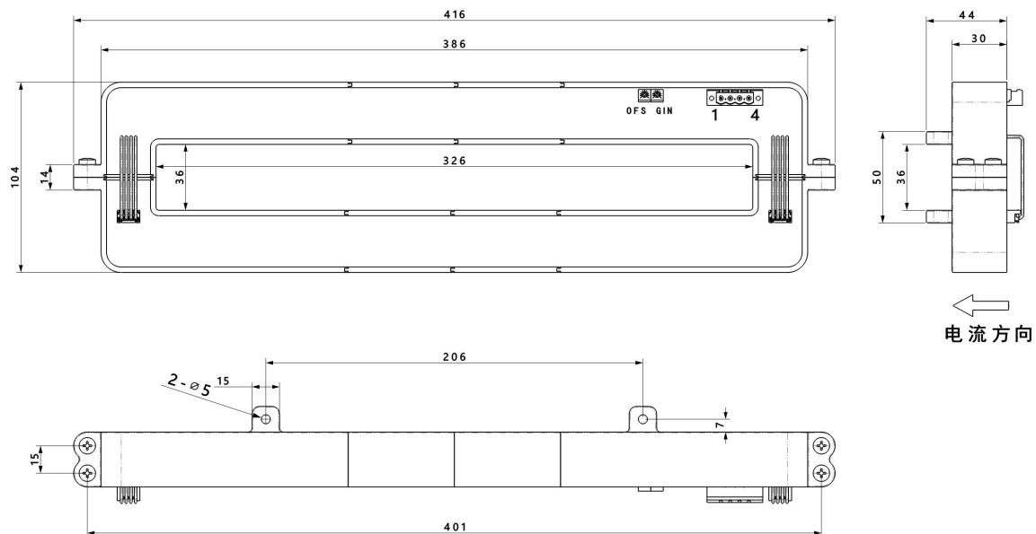
Elucidation: 1:+15V 2:-15V 3:V<sub>OUT</sub> 4:0V(GND) OFS:Zero adjustment GIN:Gain adjustment
