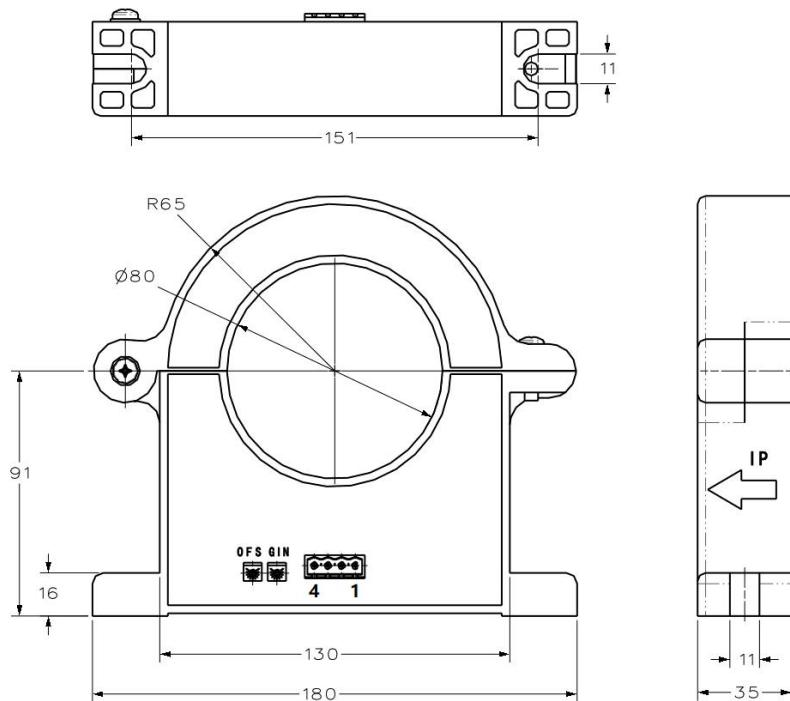
Elucidation: 1:+15V 2:-15V 3:V<sub>OUT</sub> 4:0V(GND) OFS:Zero adjustment GIN:Gain adjustment
