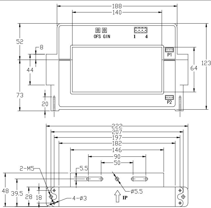
Elucidation: 1:+15V 2:-15V 3:V<sub>OUT</sub> 4:0V(GND) OFS:Zero adjustment GIN:Gain adjustment
