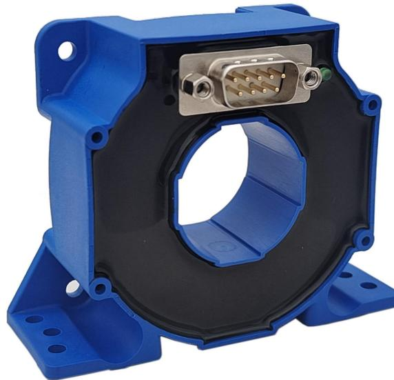
DCSM500LFBH-DB9 Current Transducer using the principle of fluxgate. It can measure DC, AC, pulse, and various irregular wave form currents under electrical isolation conditions. It has ultra-high accuracy and linearity features, ultra-high sensitivity and resolution, as well as extremely low offset current and temperature drift. It is widely used in instruments and meters, medical equipment, measurement and calibration, laboratories, high-precision power supplies, new energy vehicles.
