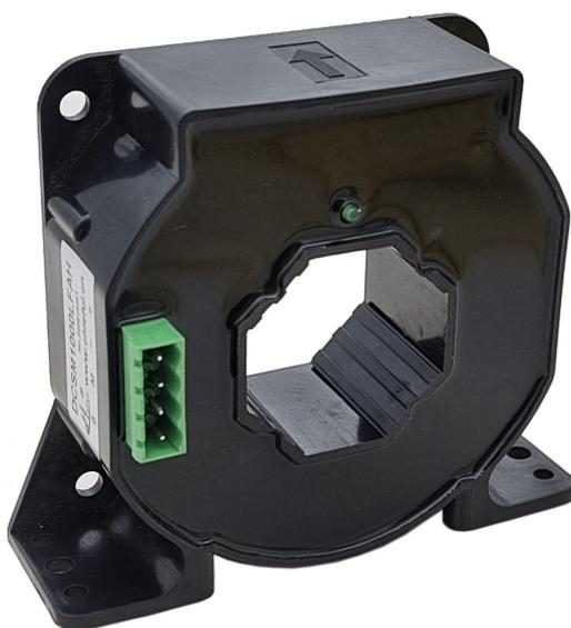
DCSM1000LFAH Current Transducer using the principle of fluxgate. It can measure DC, AC, pulse, and various irregular wave form currents under electrical isolation conditions. It has ultra-high accuracy and linearity features, ultra-high sensitivity and resolution, as well as extremely low offset current and temperature drift. It is widely used in instruments and meters, medical equipment, measurement and calibration, laboratories, high-precision power supplies, new energy vehicles.
