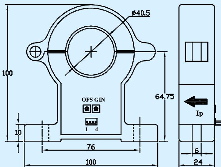
Elucidation: 1:+15V 2:-15V 3:V<sub>OUT</sub> 4:0V(GND) OFS:Zero adjustment GIN:Gain adjustment
